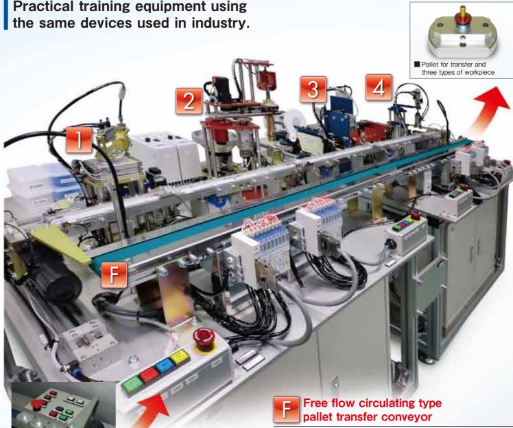
It is a transfer line in which pallets with workpieces on circulates on a belt conveyor. The pallets are detected by a transmission type photoelectric sensor and positioned at each station. After the workpieces assembled on a pallet are moved outside the line, an empty pallet will return to the top position by a return conveyor.
